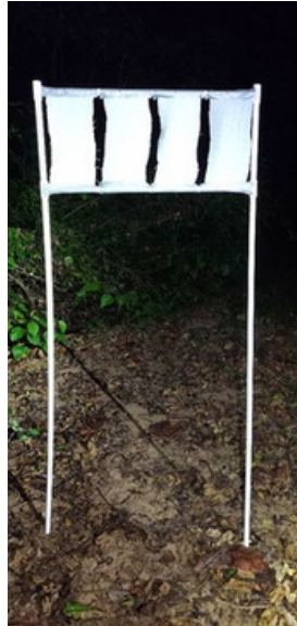
Deployed passive air filters.
